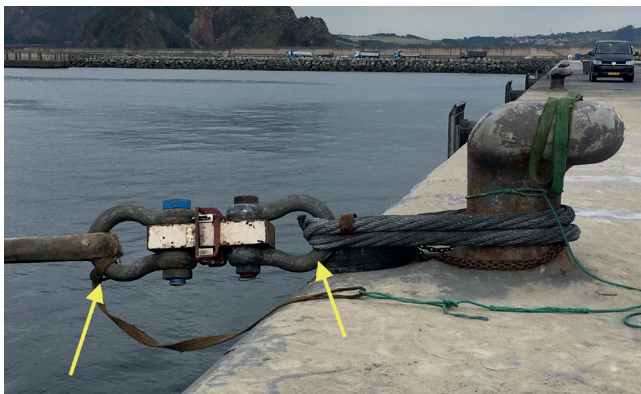
Figure 3: asymmetrical load distribution through load cell due to misalignment from towline
