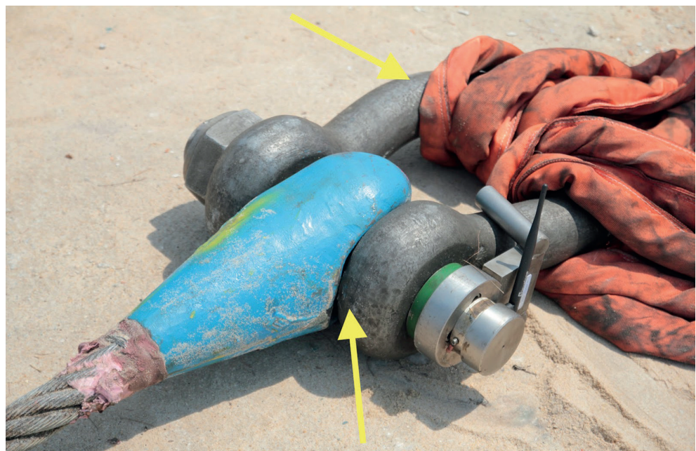
Figure 3: asymmetrical load distribution through load cell due to misalignment from towline
